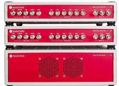
Two oscillation controllers (Dual-OC4) digitally integrated with the Nanonis real-time controller. The two OC4 devices can be used either as two PLLs or two lock-in detectors, or one PLL and one lock-in.
