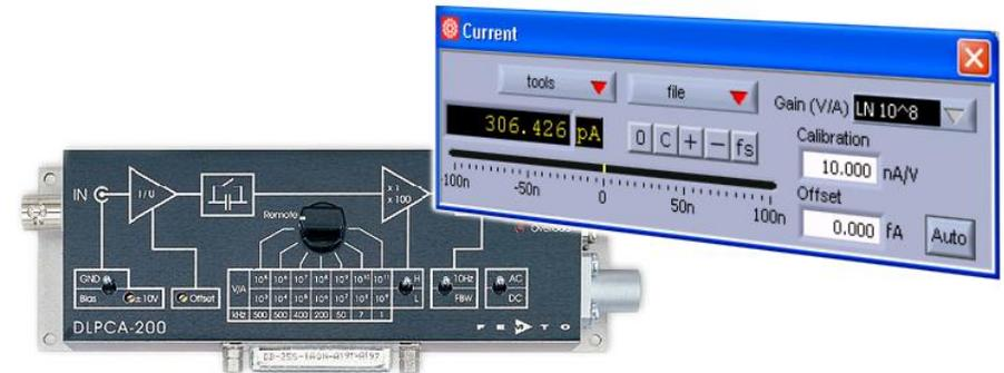
The preamplifier is powered from the Nanonis SC4 and controlled via digital lines that set gain and bandwidth and take care of the correct current calibration.
